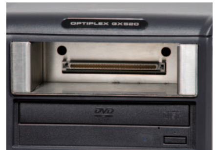
Copy module made from stainless steel in combination with the steel back side of the CardBoxes prevents electrostatic discharge
